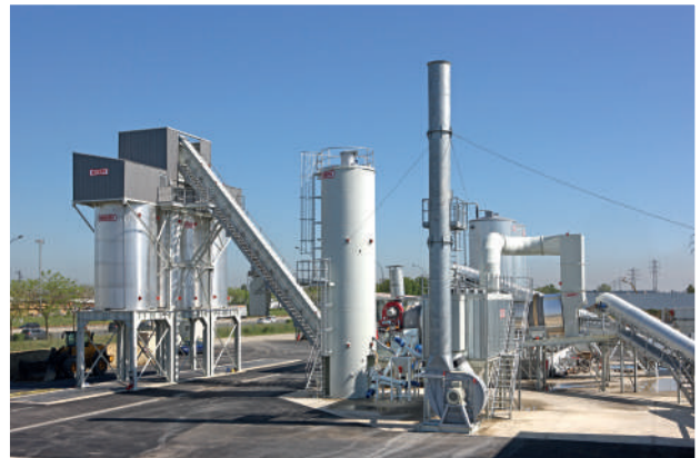
Silos with drag conveyor.
