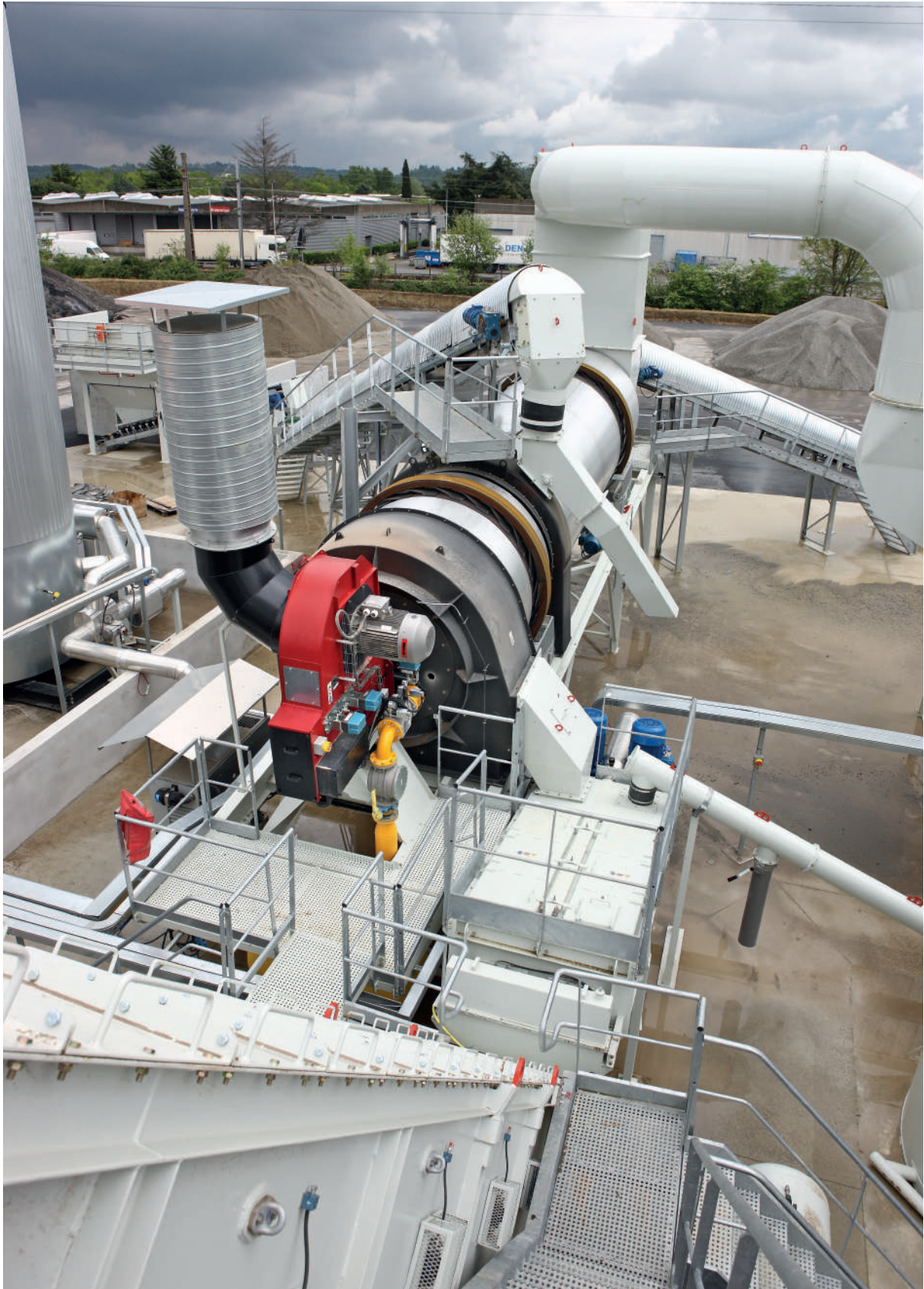
Dryer and mixer of a continuous Flow-Mix 220.
