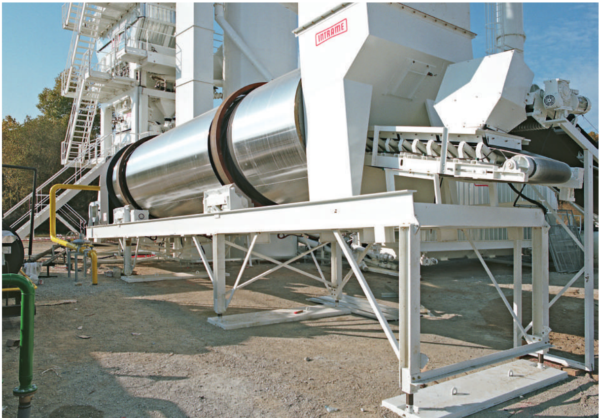
Detail of dryer's load distributors.
