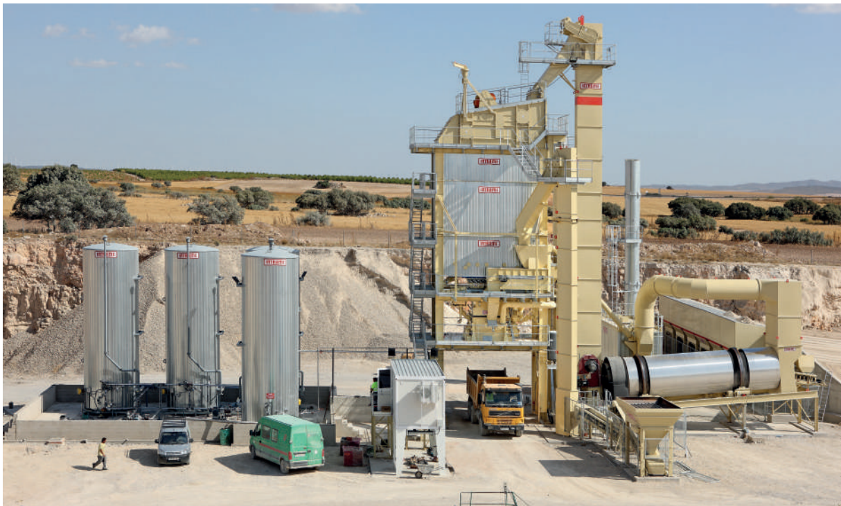
280 t/h asphalt plant (Spain). With InNOVA-G mixing tower. Equipped with 160 t capacity hot bins. Bitumen and fuel tanks electrically heated. 4.500 kg mixer. Equipped with cold process recycling system unloading in the mixer.
