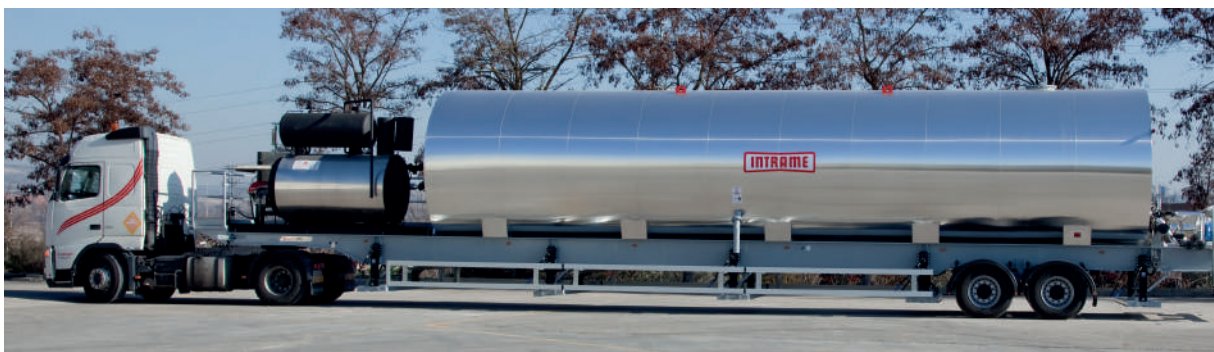
Mobile tank on wheels incorporating heater.
