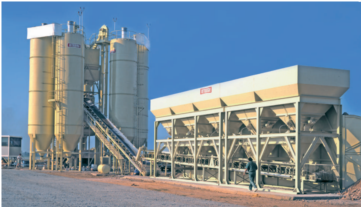
Concrete plant PH-150 equipped with a 3 m 3 twin shaft horizontal mixer working at Barcelona's airport.
