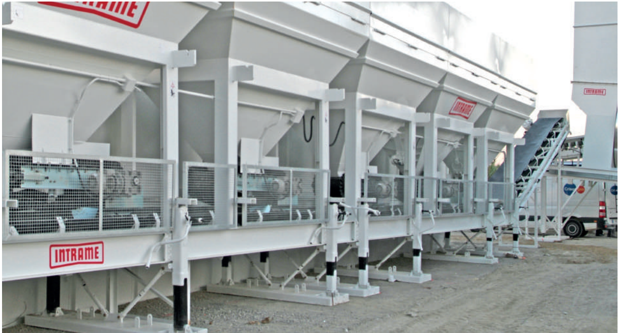
Detail of cold feeders load distributors.
